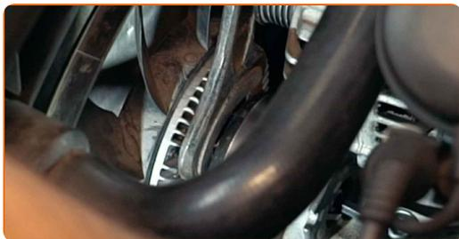
**23** Loosen the alternator fasteners. Use HEX No.H8.
