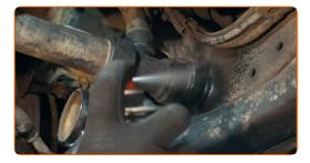
Disconnect the coolant pipe retaining clip.
