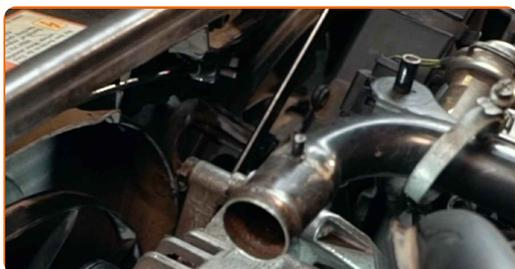
**44** Remove the coolant reservoir cap.
