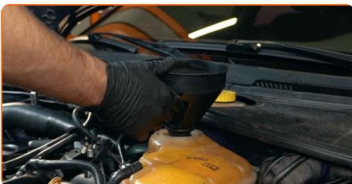
**46** Pour coolant in the coolant reservoir.
