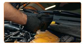
Pour coolant in the coolant reservoir.
