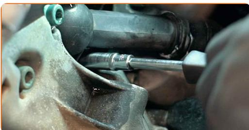
**29** Remove the thermostat housing.
