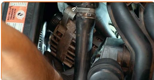
**25** Disconnect the alternator connector.
