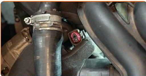
**26** Unscrew the alternator power cable fastener. Use a combination spanner #13.
