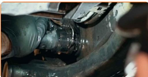
**13** Connect the coolant pipe retaining clip.
