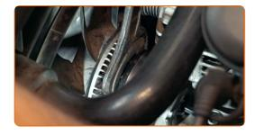
Loosen the alternator fasteners. Use HEX No.H8.
