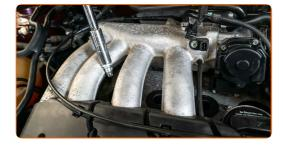
Screw new spark plugs and tighten them. Use a torque wrench. Use the spark plug socket #16. Tighten it to 25 nm torque.
