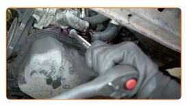
Remove the thermostat housing.
