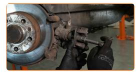
Treat the back side of the new brake pads. Treat the brake caliper bracket where it contacts the brake pads. Use anti-squeal paste.
