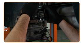
Remove the brake caliper.
