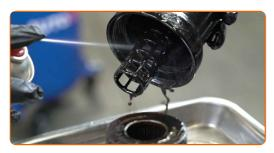
Install a new 0-ring to its mounting seat on the filter cover.
