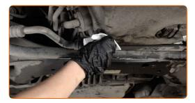
Screw in the new drainage plug and tighten it. Use a drive socket #19. Use a torque wrench. Tighten it to 26 Nm torque.
