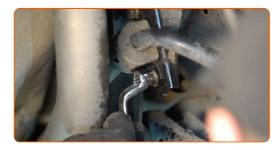
Unscrew the fasteners connecting the stabiliser link to the stabiliser bar. Use a combination spanner #15. Use a drive socket #15. Use a ratchet wrench.
