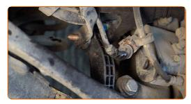
Screw the fasteners of the stabilizer bush brackets. Use a combination spanner #15. Use a drive socket #15. Use a torque wrench. Tighten it to 35 Nm torque.
