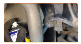
Unscrew the fasteners of the stabilizer bush brackets. Use a combination spanner #15. Use a drive socket #15.
