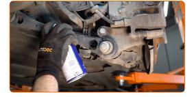
Unscrew the fastener connecting the stabilizer link to the control arm. Use a drive socket #15.
