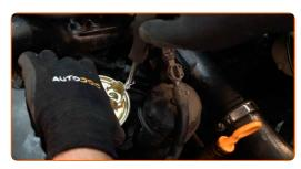
Remove the o-rings. Use a flat screwdriver.
