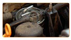
Disconnect the pipe from the fuel filter.
