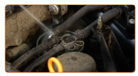
Loosen the fastening clamps of the fuel filter pipes. Use hose clamp pliers with retainer.
