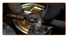
18 Install the fuel filter pipe retainer.
