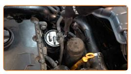
10 Remove the fuel filter pipe retainer.
