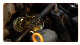
Attach the tubes to the fuel filter.
