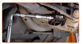
16 install the rod fastening to the stabilizer and tighten it. Use a combination spanner #15. Use a drive socket #15. Use a torque wrench. Tighten it to 55 Nm torque.
