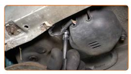
Remove the oxygen sensor housing cover.
