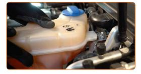
Screw in the coolant reservoir fasteners. Use Torx T25.
