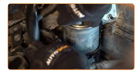
Remove the o-rings. Use a flat screwdriver.
