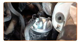
Attach the pipe to the fuel filter.
