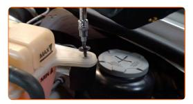
Remove the coolant reservoir.
