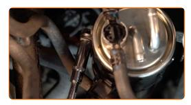
Disconnect the pipe from the fuel filter.
