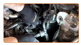
Tighten the fastening clamp of the fuel filter pipe. Use clic-R collar pliers.
