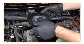
Pour coolant in the coolant reservoir.
