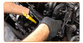
Tighten the fastener of the secondary air pump bracket. Use HEX No.H6. Use a drive socket #13. Use a torque wrench. Tighten it to 9 Nm torque.
