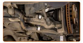
Tighten the fastener connecting the stabilizer link to the stabilizer bar. Use a combination spanner #16. Use a torque wrench. Tighten it to 40 Nm torque.+90°
