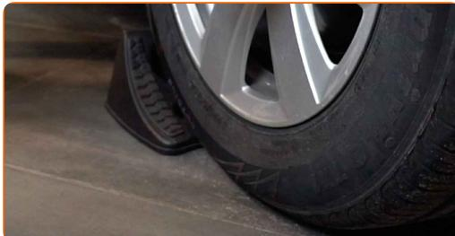
**3** Loosen the wheel hub fastener. Use HEX No.H16. Use a tap wrench.
