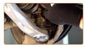
Install the fastening bolt. Use a combination spanner #21.
