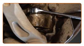
Disconnect the ball joint from the steering knuckle. Use a ball joint puller.
