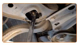
Remove the fastening bolt. Use a crowbar.
