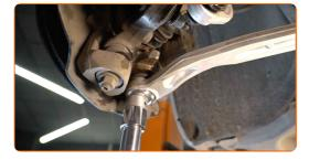
Screw the rear fastener connecting the control arm to the subframe. Use a combination spanner #18. Use a drive socket #18. Use a torque wrench. Tighten it to 70 Nm torque.+180°
