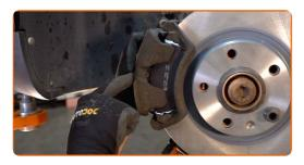
Connect the brake pads wear sensor.
