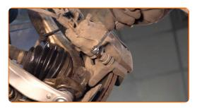
Disconnect the brake pads wear sensor. Use a crowbar.
