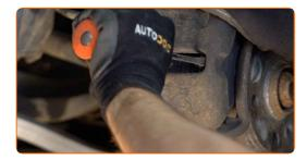
11 Remove the brake caliper.
