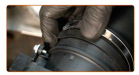
6 Undo the fastening screws of the air filter cover. Use Torx T30. Use a ratchet wrench.
