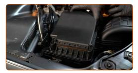
Screw in the fastening screws of the air filter cover. Use Torx T30. Use a ratchet wrench.
