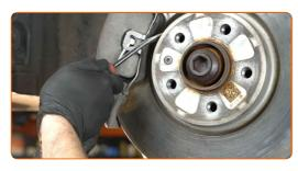
11 Remove the brake caliper.
