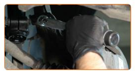
19 Install the brake caliper retaining spring.
