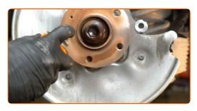
20 Install the brake disc.
