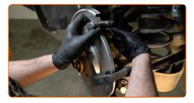
Tighten the brake caliper bracket. Use a drive socket #18. Use a torque wrench. Tighten it to 100 Nm torque.+90°
