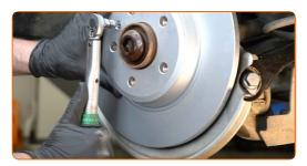
Remove the retaining springs of the brake pads.
