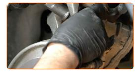
Install the retaining springs of the brake pads.
