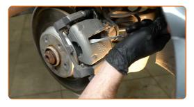
11 Remove the brake caliper.
