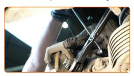
15 Remove the caliper bracket.
