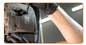
Detach the brake caliper retaining spring. Use a crowbar. Use a flat screwdriver.
