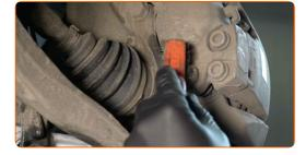
Unscrew the brake caliper fastening. Use a drive socket #13. Use a ratchet wrench.
