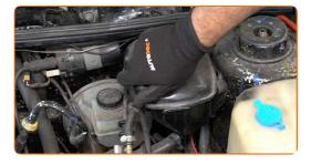
Remove the fender protection cover.
