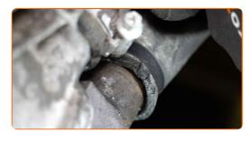
Drain the coolant from the engine.
