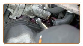
9 Remove the thermostat housing.
