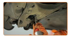
Tighten the fastener connecting the stabilizer link to the stabilizer bar. Use a combination spanner #16. Use a combination spanner #18. Use a torque wrench. Tighten it to 45 Nm torque.
