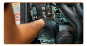
Tighten the alternator fasteners. Use HEX No.H8. Use a torque wrench. Tighten it to 8 nm torque.
