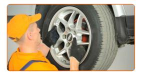
Replacement: brake caliper – AUDI A4 Saloon (8E2, B6). Tip:
