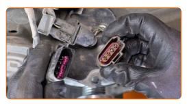
Disconnect the oxygen sensor wiring.
