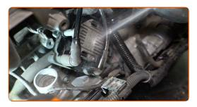
5 Disconnect the spark plug wires from the ignition coil.
