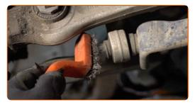
Unscrew the fastener connecting the stabilizer link to the stabilizer bar. Use a combination spanner #16 (2 pieces).
