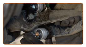
Tighten the fastener connecting the stabilizer link to the stabilizer bar. Use a combination spanner #16. Use a drive socket #16. Use a torque wrench. Tighten it to 40 Nm torque.+90°
