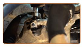
Remove the fastening bolt. Use a flat metal-working chisel. Use a hammer.
