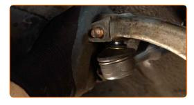
Screw on the fastening nut that connects the tie rod end to the steering knuckle. Use a drive socket #13. Use a ratchet wrench.
