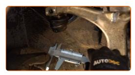
Loosen the lock nut securing the tie rod end to the tie rod. Use a combination spanner #18. Use a combination spanner #22.
