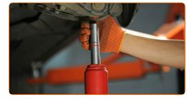
11 Remove the fastening bolt.
