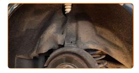
Install and tighten the wheel arch cover fasteners. Use Torx T25.
