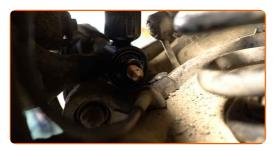
Screw in the lower fastener of the shock absorber. Use a combination spanner #21. Use a drive socket #21. Use a ratchet wrench.
