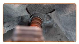
Unscrew the upper fastener of the shock absorber. Use a drive socket #13. Use a ratchet wrench.
