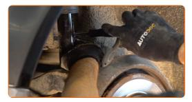
Remove the support from under the arm.
