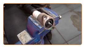
Screw the shock strut piston rod upper fastening. Use a shock absorber socket DDNº6. Use a drive socket #16. Use a torque wrench. Tighten it to 25 Nm torque.
