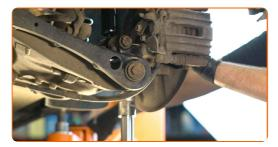
Tighten the lower fastener of the shock absorber. Use a combination spanner #21. Use a drive socket #21. Use a torque wrench. Tighten it to 150 Nm torque.+90°
