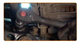
9 Remove the fastening bolt.
