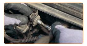
6 Unscrew the brake fluid reservoir cap.
