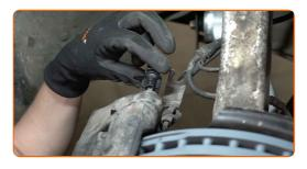
Connect the brake pad wear sensor plug.
