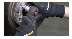
Remove the brake disc.
