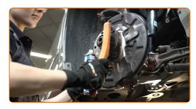
22 Install the brake disc.
