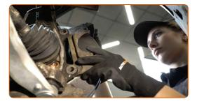
Tighten the brake caliper bracket. Use a drive socket #21. Use a torque wrench. Tighten it to 190 Nm torque.
