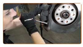
Remove the brake caliper.
