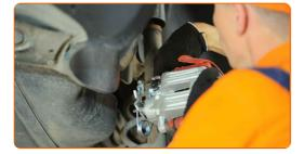
Undo the brake bleeder screw. Use a flare nut spanner #10.
