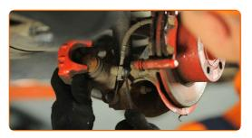
14 Remove the brake pads.
