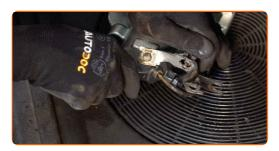
Secure the brake hose fastening bracket. Use a drive socket #11. Use a ratchet wrench.
