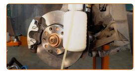
Undo the brake bleeder screw. Use a combination spanner #10.
