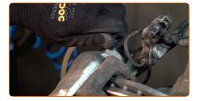
Tighten the brake caliper bleed screw. Use a drive socket #10. Use a torque wrench. Tighten it to 9 Nm torque.
