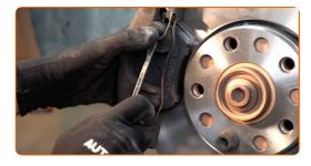
Remove the brake caliper.
