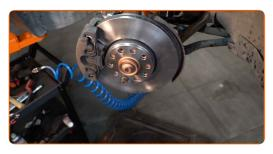
Clean the brake pipe fastener. Use a wire brush. Use a brake cleaner.
