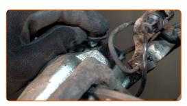
Bleed the brake caliper system. Without starting the engine, press the brake pedal several times until you feel significant resistance.
