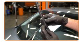
Remove the blade from the wiper arm.
