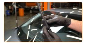
Remove the blade from the wiper arm.
