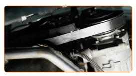
Return the tensioner pulley to its initial position. Use a combination spanner #16.
