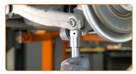
Tighten the fastener connecting the stabilizer bar with the control arm. Use a combination spanner #16. Use a drive socket #16. Use a torque wrench. Tighten it to 40 Nm torque.+90°
