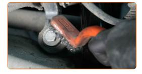
Unscrew the fastener connecting the stabilizer bar with the control arm. Use a drive socket #16. Use a ratchet wrench.
