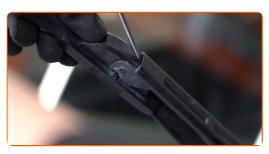
Remove the blade from the wiper arm.
