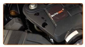
Unscrew the engine cover fastener. Use a drive socket #10.
