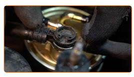
18 Install the fuel filter pipe retainer.
