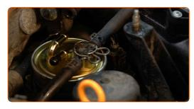
Attach the tubes to the fuel filter.
