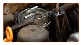
Disconnect the pipe from the fuel filter.
