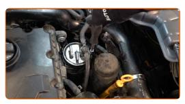
10 Remove the fuel filter pipe retainer.
