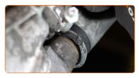
Drain the coolant from the engine.
