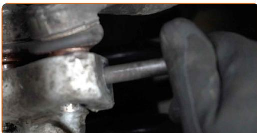
**11** Detach the upper control arm from the steering knuckle. Use a flat metal-working chisel. Use a hammer.
