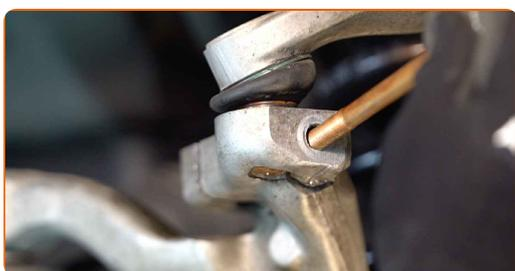
**42** Tighten the upper arm fastenings. Use a combination spanner #16. Use a drive socket #16. Use a torque wrench. Tighten it to 40 Nm torque.
