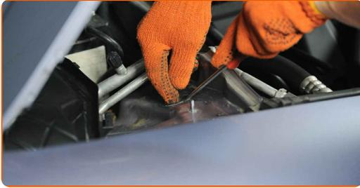
**19** Unscrew the upper fasteners of the shock strut. Use a drive socket #16. Use a ratchet wrench.
