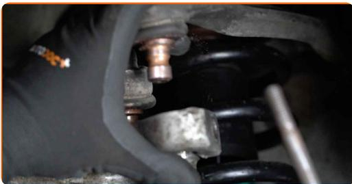
**12** Detach the bottom part of the shock strut.
