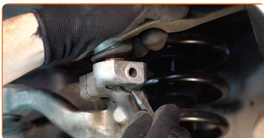
**41** Install the fastening bolt. Use a hammer. Use a pin punch.
