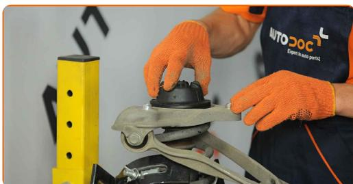
**27** Tighten the shock strut piston rod nut. Use a drive socket #18. Use a ratchet wrench. Use a torque wrench. Tighten it to 50 Nm torque.
