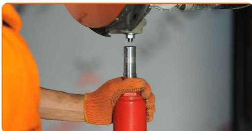
**45** Tighten the lower fastening of the shock absorber. Use a combination spanner #18. Use a drive socket #18. Use a torque wrench. Tighten it to 90 Nm torque.
