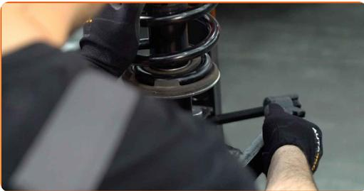
**30** Install the shock strut into the wheel arch.
