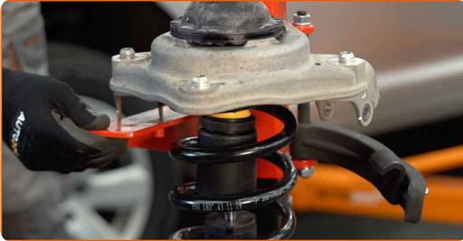
**29** Remove the assembled shock strut.
