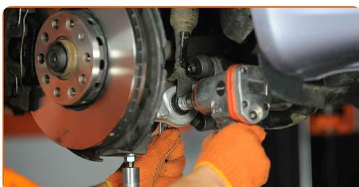
**46** Remove the support from under the steering knuckle.
