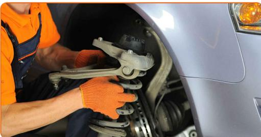
**31** Secure the upper fasteners of the shock strut.
