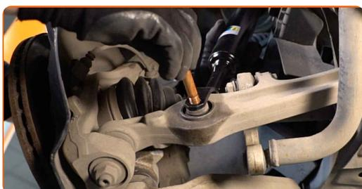
**44** Prop up the steering knuckle. Use a hydraulic transmission jack.
