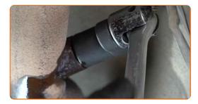
Remove the oxygen sensor.
