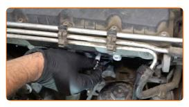
Tighten the glow plugs. Use the spark plug socket #10. Use a torque wrench. Tighten it to 15 nm torque.
