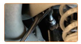
Unscrew the fastener connecting the control arm to the rear knuckle. Use a drive socket #18. Use a ratchet wrench.
