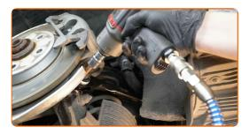
Screw the fastener connecting the control arm to the subframe. Use a combination spanner #18. Use a drive socket #18. Use a ratchet wrench.
