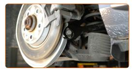
Remove the support from under the arm.
