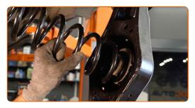
Support the arm. Use a crowbar. Use a hydraulic transmission jack.
