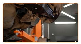
Tighten the arm fastening to the beam. Use a combination spanner #18. Use a drive socket #18. Use a torque wrench. Tighten it to 95 Nm torque.
