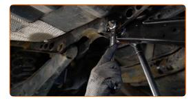
Tighten the fasteners connecting the control arm to the rear knuckle. Use a combination spanner #18. Use a drive socket #18. Use a torque wrench. Tighten it to 90 Nm torque.+90°
