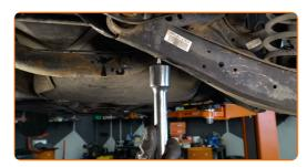
Loosen the fastener that connects the control arm to the rear knuckle. Use a combination spanner #18. Use a drive socket #18. Use a ratchet wrench.
