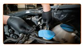
Detach the bulb holder by turning it by  $\sim 30^\circ$ . Remove the holder from the headlight mounting seat.
