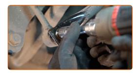
Unscrew the fastener connecting the stabilizer link to the control arm. Use a drive socket #15. Use a ratchet wrench.
