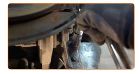
install the rod fastening to the stabilizer and tighten it. Use a combination spanner #14. Use XZN #6. Use a drive socket #15. Use a torque wrench. Tighten it to 45 Nm torque.
