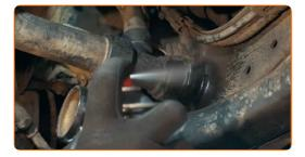
Disconnect the coolant pipe retaining clip.
