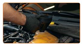
Pour coolant in the coolant reservoir.
